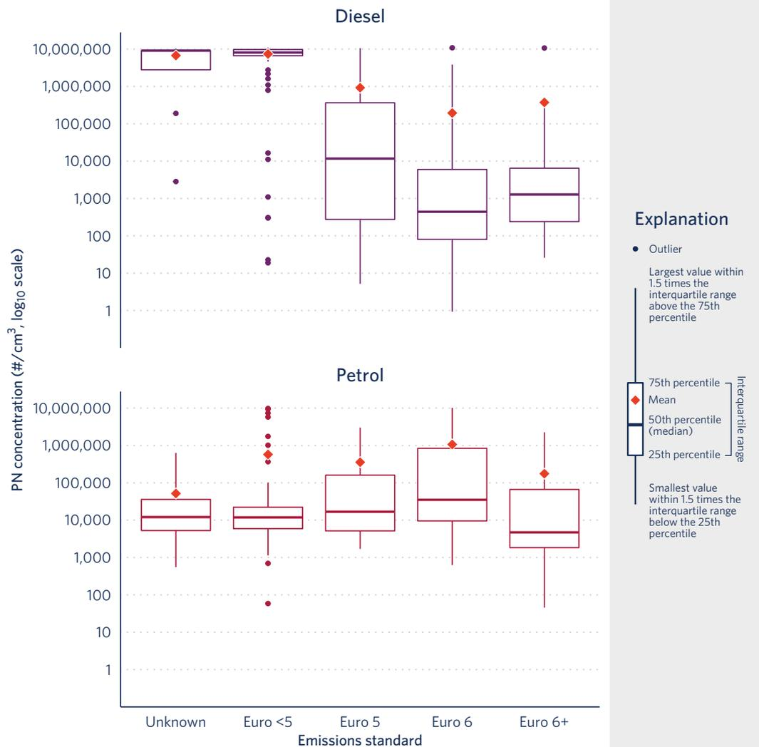
Boxplot of PN tailpipe emission concentration of light-duty vehicles by Euro standard and fuel type. Diamonds represent the mean emissions. “Euro 6+” refers to Euro 6d-TEMP and Euro 6d. The proposed particle number limit for periodic technical inspection programs in Belgium currently applies to Euro 5b and higher DPF-equipped vehicles. A limit for diesel Euro 5a vehicles is still under discussion.
