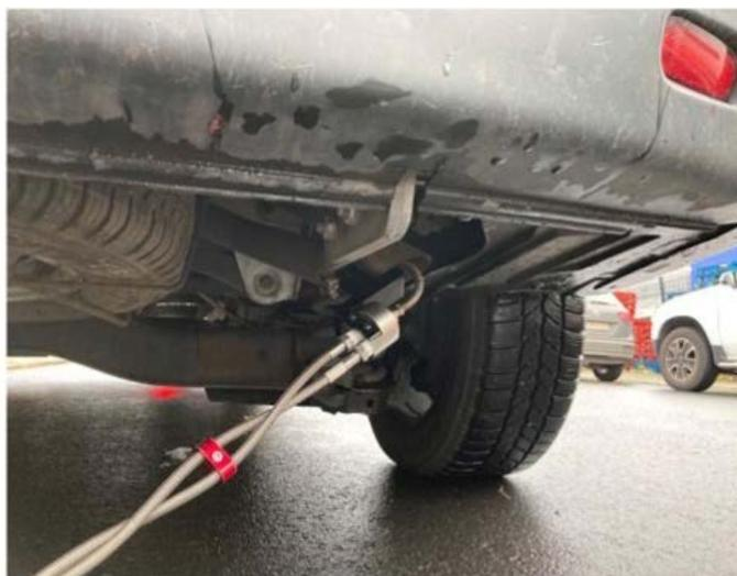
Roadside remote-sensing emission testing including PM measurement (left) and particle number inspections using a portable emission tester (right) on Rue du Lieutenant Lotin, Brussels
