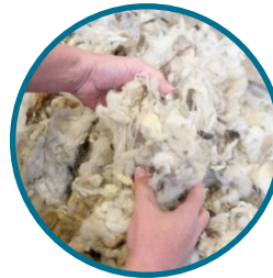
Schapenwol in bulk \lambda = 0,041 \text{ W/mK}
