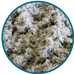
Cellulose \lambda \approx 0,038 \text{ W/mK}
