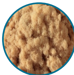
Houtvezels in bulk \lambda = 0,038 \text{ W/mK}
