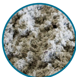
Cellulose \lambda \approx 0,038 \text{ W/mK}
