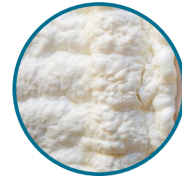
Polyurethaan \lambda \approx 0,026 \text{ W/mK}
