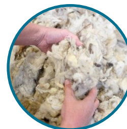
Schapenwol in bulk \lambda = 0,041 \text{ W/mK}
