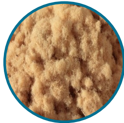
Houtvezels in bulk \lambda = 0,038 \text{ W/mK}
