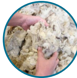
Schape wol in bulk \lambda = 0,041 \text{ W/mK}
