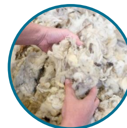
Schapenwol in bulk \lambda = 0,041 \text{ W/mK}
