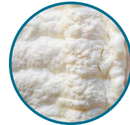
Polyurethaan \lambda \approx 0,026 \text{ W/mK}
