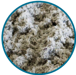
Cellulose \lambda \approx 0,038 \text{ W/mK}
