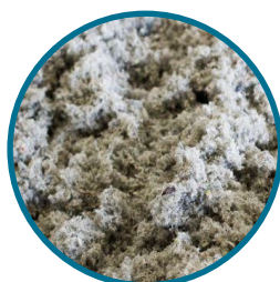
Cellulose \lambda \approx 0,038 \text{ W/mK}
